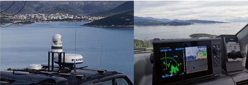
Fig. 30.3 Photographs of the surveillance equipment installed in the HCG patrol van
