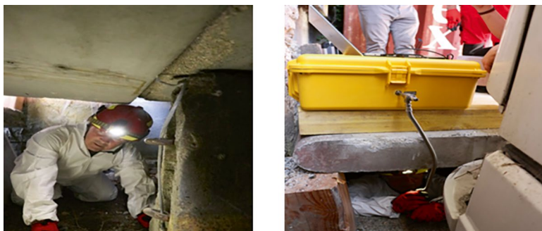
Fig. 7.1 Testing of the RESCUE-MIMS in the field under the scenario “People Trapped Under the Rubbles” that took place in Limoges, France in cooperation with the PUI team
