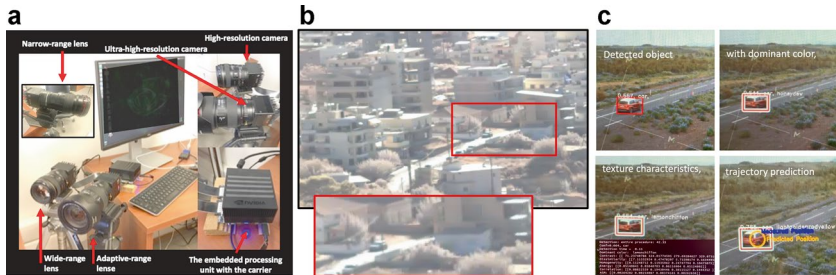
Fig. 32.6 HW setup of the high-resolution optical sensor (a). Examples of target detection in the horizon (1 km distance) direction (b) and tracking and characterization of target (c)
