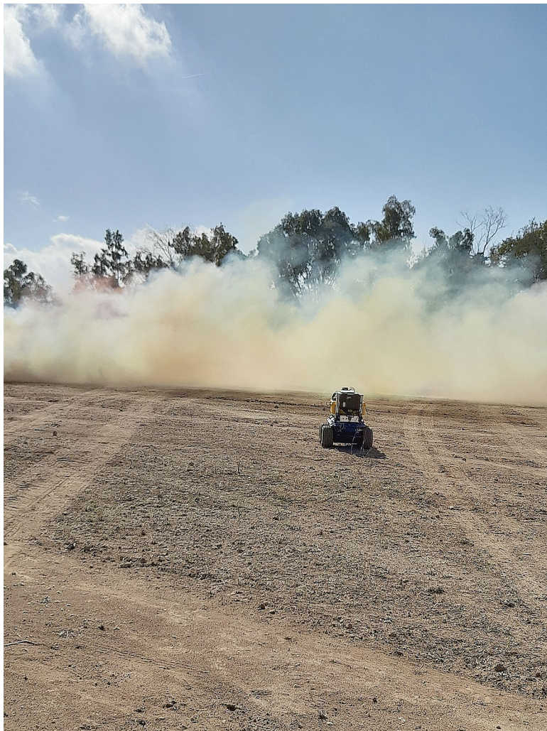
Fig. 7.2 The RESCUE-MIMS on-board the SeekurJr robotic platform by DFKI was used as a remote early warning system of a hazardous smoky environment for the first responders
